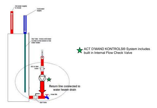
Your ACT D'MAND KONTROLS<sup>®</sup> System has <sup>3</sup>/<sub>4</sub>" male pipe thread fittings (MPT) on either side of the pump which will need to be adapted to the existing plumbing line. Pipe sealant or Teflon tape is recommended to ensure there are no leaks. Once the unit is plumbed in to the return line you can then proceed to connecting the controllers.
