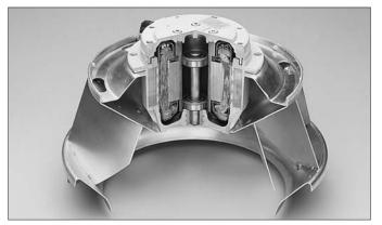
All FKD Series fans are powered by an external rotor motorized impeller. This design provides excellent heat dissipation even at low rpm. All of the FKD Series fans are 100% speed controllable through voltage reduction allowing for precision balancing of systems. FKD8XL through 18 are supplied standard with 115/1/60 motors. FKD18XL and FKD20 have a standard configuration of 230-460/3/60. For additional motor options please contact Fantech Technical Support at 1-800-747-1762.
