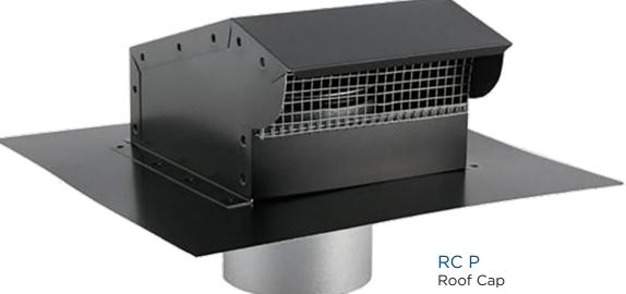
Roof Cap with backdraft damper, duct connection and screened exhaust opening. Available in 4, 5, 6, 8, 10, and 12 inch duct sizes.
