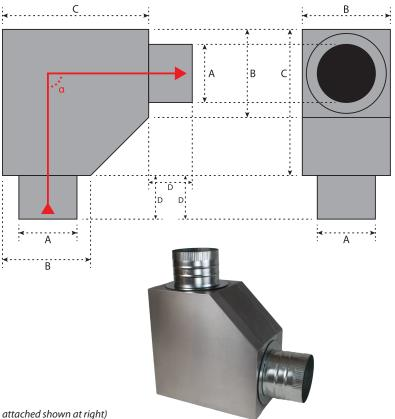
(Silencer with duct connection flanges attached shown at right)
