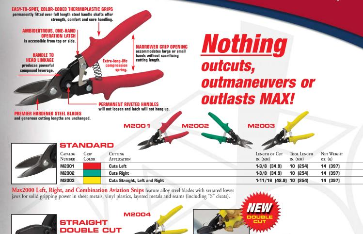
The Max2000 Double Cut Snip employs a best-of-all-worlds close tolerance design for consistent performance. A curved cutting edge on the center jaw reduces cutting force required and large relief grinds on all jaws minimize drag. The double cut blades feed smoothly, cut cleanly without surface distortion, and easily navigate metal seams encountered in round metal duct and stove pipe. A self-starting point on center jaw makes short work of blind cuts.
