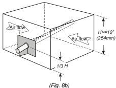
Horizontal duct with a minimum height of 10" (254mm)
