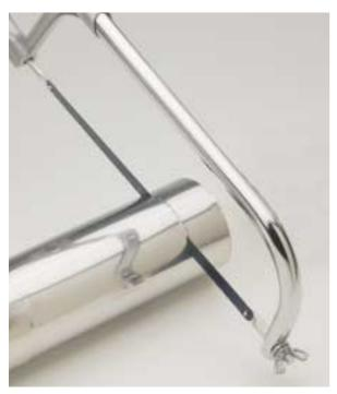
\*The lengths of pipe may be cut on non-expanded end using aviation snips or a hacksaw (24 tpi). The cut end must be filed or sanded smooth before joining.
