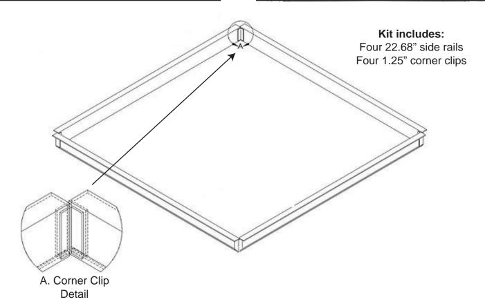
Attach the 4 side rails using the 4 corners clips.
