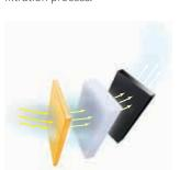
1st stage: PREFILTER filters large particulate and captures some V.O.C.s
