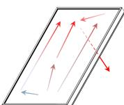
Outgoing air temperature is heated to  $22^{\circ}$  C /  $40^{\circ}$  F higher than incoming air and returned to the living space at 60-90 ft<sup>3</sup> / min
