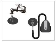
Clean the filter as often as it gets dirty, but at least 3-4 times a year. Clean the filters, let them get dry and install the dry filters inside the air duct Vacuum cleaning is allowed. The filter rated service life is 3 years.
