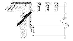
Screw holes are drilled at a 45° angle on inner flange. Only available with Removable Core.
