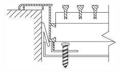
Product is fastened to duct-mounted brackets, which are concealed behind the blades.
