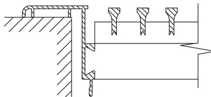
Designed for lay-in ceiling and custom applications. For lay-in, order 2" under to account for flange.
