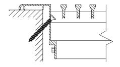
Screw holes are drilled at a 45° angle on inner flange. Only available with Removable Core.
