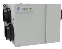
Suitable for temperate climates where balanced ventilation is needed, an Air Exchanger Ventilator (AEV 80) is designed to provide fresh air into a building while exhausting an equal amount of stale air. During the winter months, the incoming cold fresh air is warmed by mixing it with return air before it is supplied to the home. During summer months when the indoor space is air conditioned, the AEV will help in cooling the incoming fresh air with the stale air that is being exhausted.
