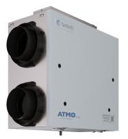
Fantech's, ATMO 150E is an Energy Recovery Ventilator designed for higher static pressure applications. The unit brings a continuous supply of fresh air into a home while exhausting an equal amount of contaminated air. The energy recovery core at the center of the unit transfers heat and moisture from incoming air to the outgoing air that was cooled and dried by the building's air conditioner.
