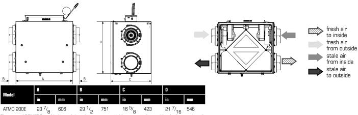
Clearance of 22" (559 mm) in front of the unit is recommended for removal of core. All units feature three foot plug-in power cord with 3-prong plug.
