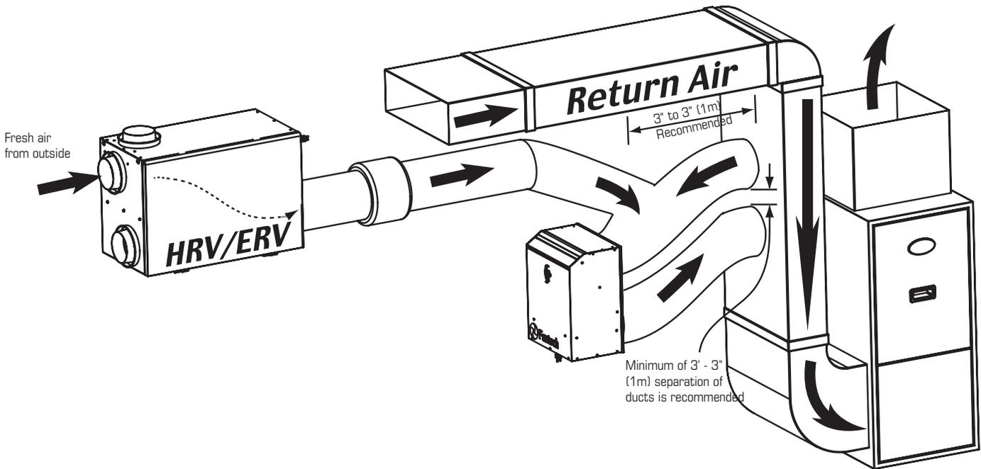
Ventilation system (HRV/ERV) should be installed and balanced in accordance with its installation manual.
