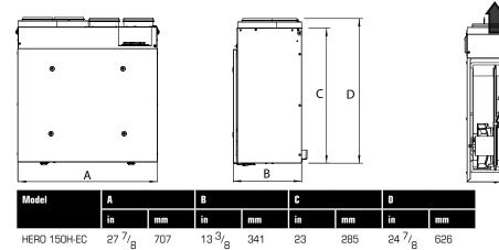
Dimensional information is in inches. Clearance of 14" (355mm) in front of the unit is recommended for removal of core. All units feature three foot plug-in power cord with 3-prong plug.
