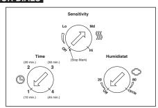
**NOTE: DO NOT** rotate the adjustment dials past the stop marks shown in the figure above.
