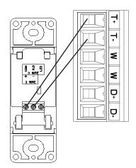
7. Re-connect the terminal connection in the HRV / ERV.
