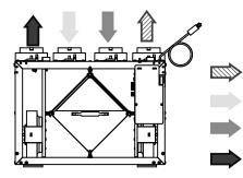
fresh air to inside fresh air from outside stale air from inside stale air to outside
