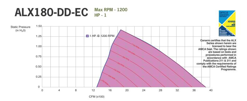
Performance certified is for installation type A- Free Inlet, Free outlet, Power rating (HP) does not include transmission losses. Performance ratings do not include the effects of appurtenances (accessories).
