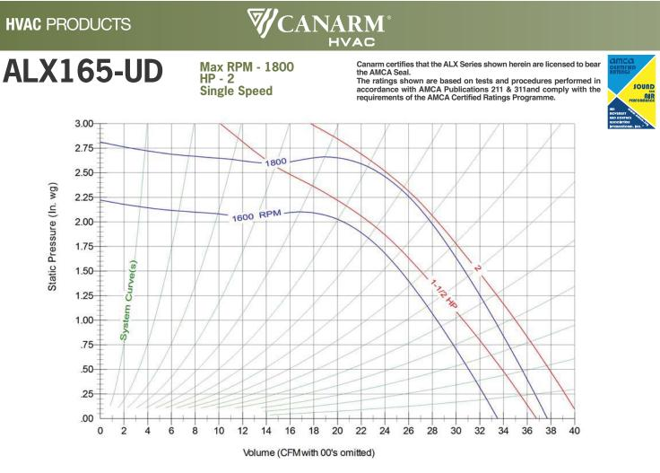
Performance certified is for installation type A- Free Inlet , Free outlet, Power rating (HP) does not include transmission losses. Performance ratings do not include the effects of appurtenances (accessories).
