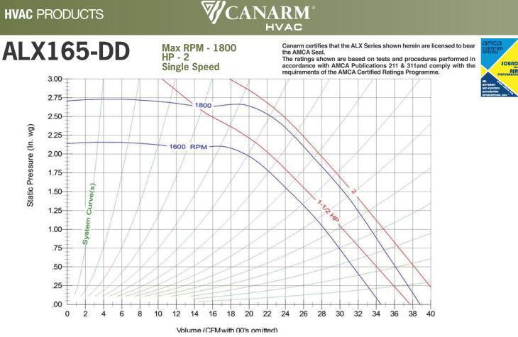
Performance certified is for installation type A- Free Inlet, Free outlet, Power rating (HP) does not include transmission losses. Performance ratings do not include the effects of appurtenances (accessories).
