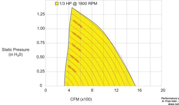
Performance certified is for installation type A- Free Inlet, Free outlet, Power rating (HP) does not include transmission losses. Performance ratings do not include the effects of appurtenances (accessories).
