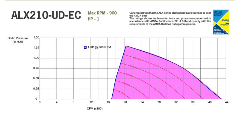
Performance certified is for installation type A- Free Inlet, Free outlet, Power rating (HP) does not include transmission losses. Performance ratings do not include the effects of appurtenances (accessories).
