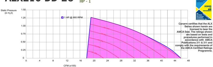
Performance certified is for installation type A- Free Inlet , Free outlet, Power rating (HP) does not include transmission losses. Performance ratings do not include the effects of appurtenances (accessories).
