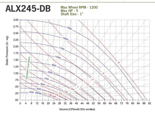
Performance certified is for installation type A- Free Inlet, Free outlet, Power rating (HP) does not include transmission losses. Performance ratings do not include the effects of appurtenances (accessories).
