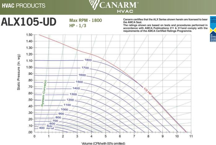
Performance certified is for installation type A- Free Inlet , Free outlet, Power rating (HP) does not include transmission losses. Performance ratings do not include the effects of appurtenances (accessories).
