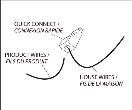
3. **WARNING: Wiring must comply with all applicable electrical codes. Turnpower OFF before removing or installing connectors.**
