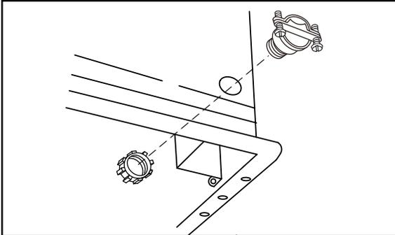
1. Secure a UL recognized or listed wire coupling or strain relief (not included) through the knock-out or hole on the casing.
