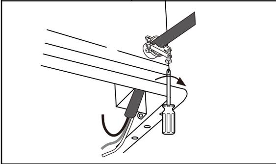
2. Install the conduit or armored cable through the wire coupling. Secure the cable by tightening the two screws on the wiring coupling.
