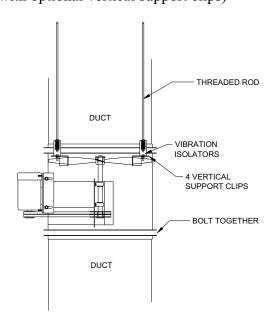
Suspended Vertically (complete with optional vertical support clips)
