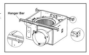
2.Extend the hanger bars to the width of the framing. Position the ventilator with the bottom edge of the hanger bar tabs are flush with the bottom edge of the framing, holding the ventilator in place. Secure hanger bars to framing using one screw on each end of hanger bar. Select a proper hole and secure the hanger bars together using one screw.
