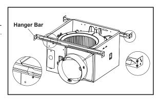
2.Extend the hanger bars to the width of the framing. Position the ventilator with the bottom edge of the hanger bar tabs are flush with the bottom edge of the framing, holding the ventilator in place. Secure hanger bars to framing using one screw on each end of hanger bar. Select a proper hole and secure the hanger bars together using one screw.
