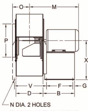
Mounting holes are 3/8" diameter on all models up to KE-11 and 9/16" on the KE-12 and KE-14.
