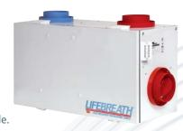
The Lifebreath® HRV allows two streams of air to pass on either side of an aluminum heat exchange core. In the winter, the core transfers heat from stale outgoing air to fresh incoming air with virtually no loss of heat to the outside. During the summer, the HRV works in reverse to keep your home cool and fresh.
