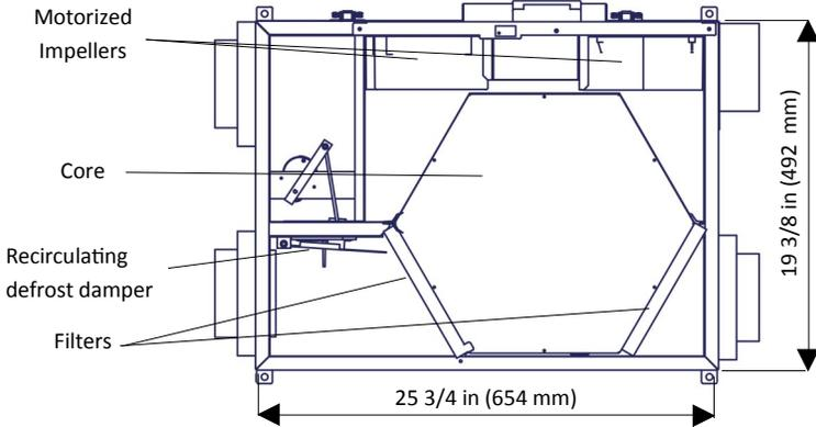
**Note:** Front clearance of 25 in (635 mm) is recommended for servicing unit. All ducts use 5 in (125 mm) round collars.
