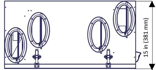
**Note:** Front clearance of 25 in (635 mm) is recommended for servicing unit. All ducts use 5 in (125 mm) oval collars, balancing dampers are located on all collars.
