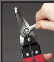
A fast adjusting, long life pivot bolt, with nylon locking nut and pressure washer, holds desired adjustment even after repetitive use in heavy gauge metal.
