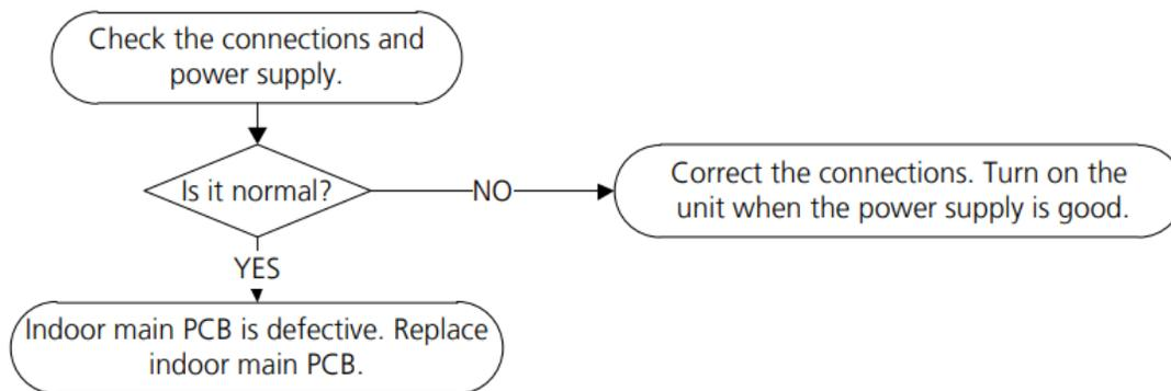
*Note: Zero crossing detection error is only valid for the unit with AC fan motor, for other models, this error is invalid.*
