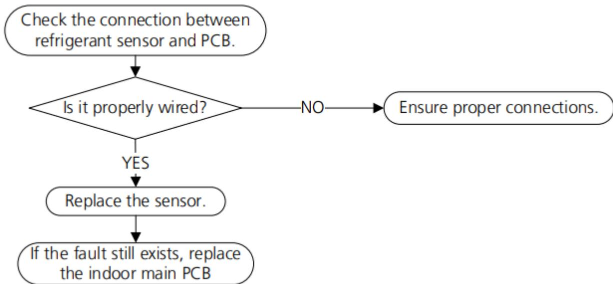
**TS06-N10: Refrigerant sensor detects leakage or refrigerant sensor is out of range and leakage is detected diagnosis and solution**
