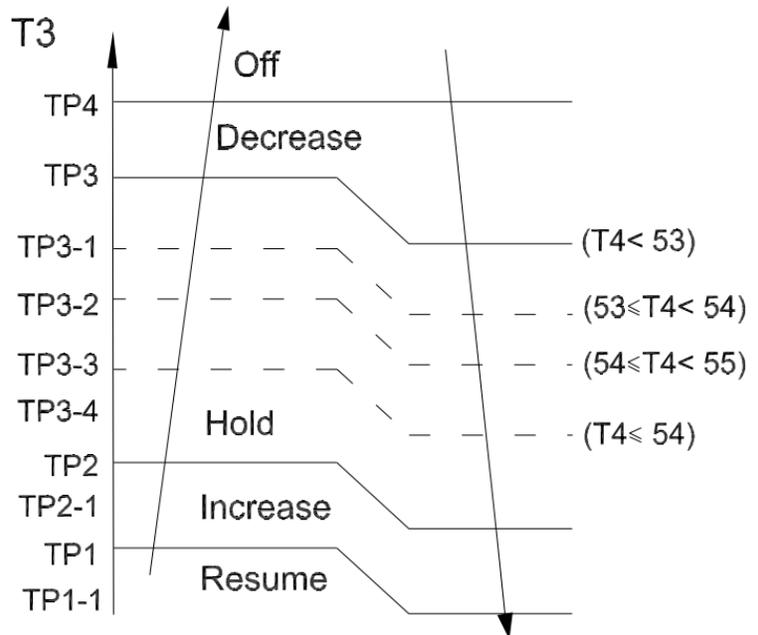
When the condenser temperature exceeds a configured value, the compressor ceases operation.
