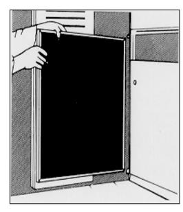
Clean monthly by rinsing your filter with running water. Particles in the ACCUMULATOR CHAMBER as well as on the electrostatic panels wash out easily through the drainage ports in the frame. For tough dirt and grease, use a mild detergent (i.e., 409 or Simple Green) and rinse thoroughly with warm water. If the filter has a directional air flow arrow label on the frame, rinse the filter by back flushing it in the opposite direction of the air flow arrow for best results.
