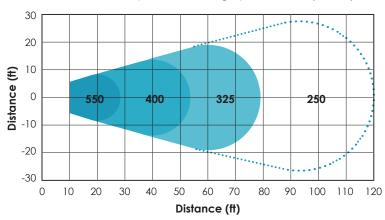
Airspeeds represent the Average velocity for each zone. Tested at 36" above floor.
