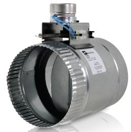
24 VAC, 1 RPM, 60 Hz, 6 Watts Maximum Torque 78 in.-oz. 2 Wire Synchronous Hysteresis Motor
