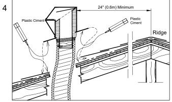
Apply plastic cement generously around the perimeter of the opening making sure to maintain a width of 4 inches. Slide the flexible duct into the opening, followed by the roof exhaust unit making sure the flashing is fully embedded in the plastic cement. Nail or screw the unit to the bridging (1 inch from the edge of the unit) while leaving a spacing of 4 inches. Finish by applying a generous amount of plastic cement to the back and sides of the flashing.
