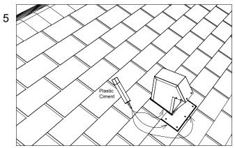
Nail the shingles in place and finish by applying a sealant around the body of the roof exhaust, flashing and shingles.
