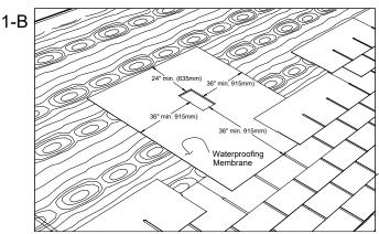
**New roof:** Install a waterproofing membrane around the opening dedicated to the installation of the roof exhaust as shown above. **Opening:** Strategically choose the location of the roof exhaust considering winter roof snow accumulations. The roof exhaust should be located in an area where snow accumulation is minimized.
