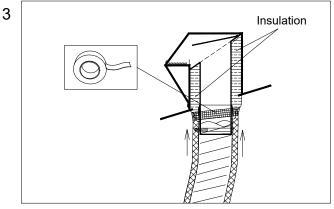
Fold the polythene (vapor barrier) over the insulation and push it to the bottom of the roof exhaust unit to ensure that the entire duct is covered. Finish by fixing it with a good quality duct tape. Ensure there are no exposed or uninsulated duct sections.
