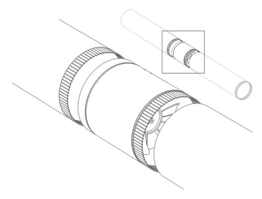
Remove a section of the existing ductwork and slide the inline fan in by slipping the duct ends over the crimped ends of the unit.
