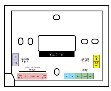
AC/DC The CO2-TH is powered from 12 to 30V AC or DC. If powering with DC +ve is applied to the top terminal and -ve is applied to the bottom terminal.
