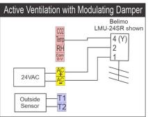
In the Installer menu you must activate the Active Ventilation function by setting the inside and outside air temperature thresholds (page 15 explains this) and defining the active ventilation output options. Once you have completed these three steps the letter "A" will be shown the in the lower right corner of the LCD to confirm the Active Ventilation function is active.
