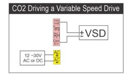
In this example a standard Variable Speed Drive is being controlled with the CO2 0-10V output. The Installer menu permits you to scale the 0-10V output to match your requirements such as output 0V at 450ppm and output 10V at 800ppm.
