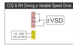
In this example the CO2 and RH is controlling the VSD with a high select. Both the CO2 and RH outputs are individually scalable so the CO2 range can be 450ppm to 1,000ppm and the RH range can be 75% to 100%. Also, the RH output can be limited to 7V max if required.
