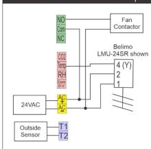
If you would like, you can have both the temperature 0-10V output and volt free relay used for advanced ventilation. In the Active Ventilation Output options menu settings select both relay and temp 0-10 (option 3). This permits you to open the fresh air damper and turn a fan on for example if outside air is suitable.
