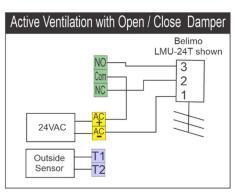
If selected in the Active Ventilation options menu, the monitor will modulate the temperature 0-10V output so that the output is at the maximum voltage set when the room temperature is 1 degree above the inside temperature setpoint. If introducing outside air the icon "A" will flash on the LCD. Tapping the "A" icon will briefly show the outside air temperature.
