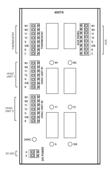
Only identical furnaces should be twinned in order to help insure that both furnace fans start at the same time.
