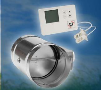
The MD6-ES24VK from S&P allows fresh air to enter dwellings to meet building code and ventilation standards requirements through a 6" motorized damper controlled by a 24V temperature/humidity monitoring control. The control can command the central HVAC blower to help distribute fresh air through the existing duct work if necessary.
