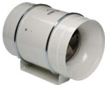
**Low profile** mixed flow fans, manufactured in plastic material (up to model 200) or in **galvanized steel** sheet protected with Epoxy paint (model 250 and 315), with external terminal box, removable motor-impeller assembly and adjustable single-phase motor, Class B, IP44.
